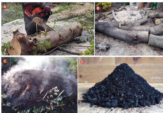
Figure 2: (a). Cutting down of the wood (b). Processing into smaller logs (c). Conventional Carbonization Chamber (d). Biochar Product of Carbonization
