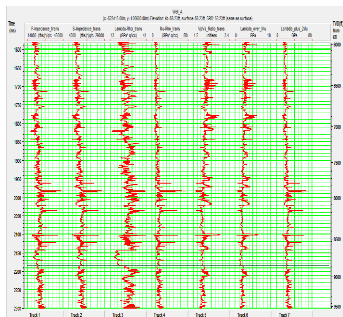
Figure 2: Well log suite showing some transformed Logs with delineated gas sand (in black rectangle).
