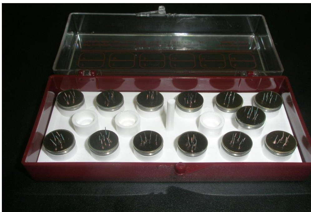
Figure 7: Photograph of hollow-fine fibres mounted on stubs for SEM analysis.
